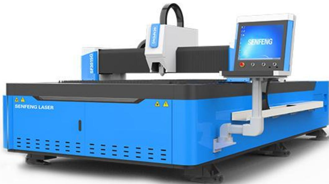
SF3015G fiber laser cutter reaches the top level in China, which is customers' best choice in metal industry. The bed is welded by precise welding process after annealing and aging treatment, and the beam is airborne aluminium castings. For the more, the running speed of the machine can reach 80 m/min.
